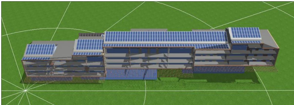
Figure 3-8: Virtual 3D Recreation of BIPV in Spanish Demo Building. Source: CENER (PV SOL)
