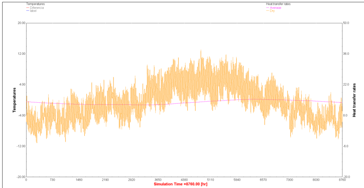
Figure 3-14: Ground Temperature-Outdoor Temperature Comparative in Dilar. Source: Trnsys-CENER
