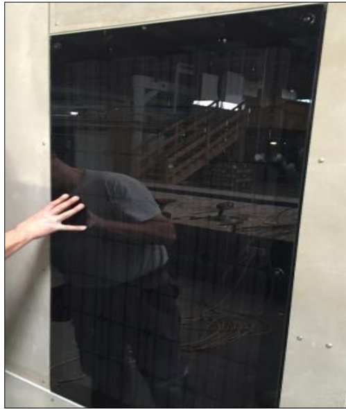
Figure 4-8: Example of an experimental integration of a photovoltaic element in a test-facade during the project HVACviaFACADE. Source: [31]
