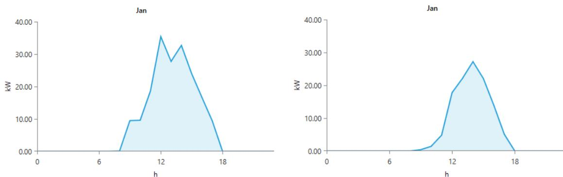
**Figure 2-4. Grid sales daily profile (kW) in January: a) PV case, b) PV+BESS case**
