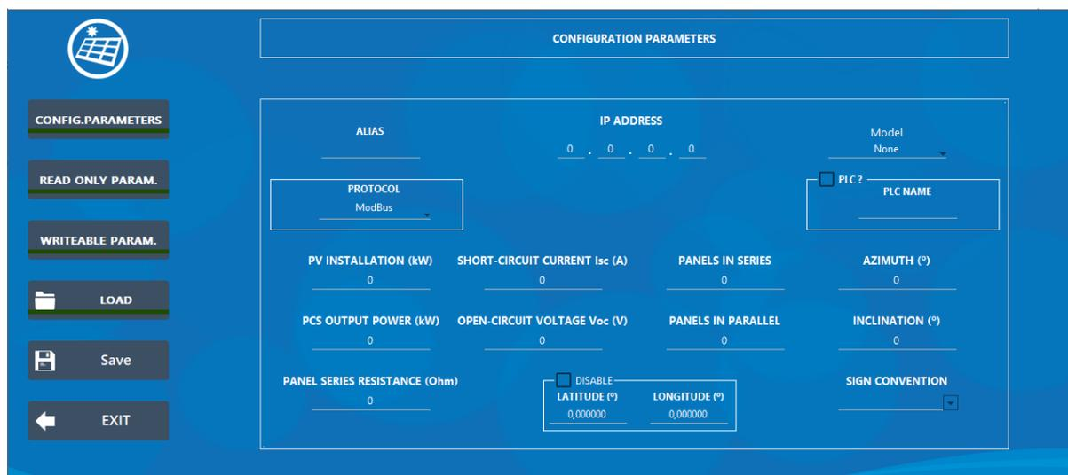
Figure 4-4. Configuration screen for an element in the SCADA
