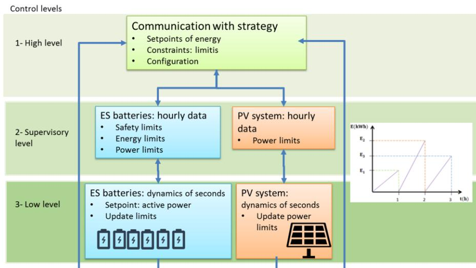
**Figure 3-1. Hierarchical control with different levels**
