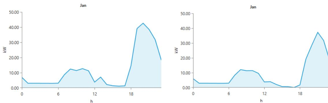
**Figure 2-3. Grid purchases daily profile (kW) in January: a) PV case, b) PV+BESS case**
