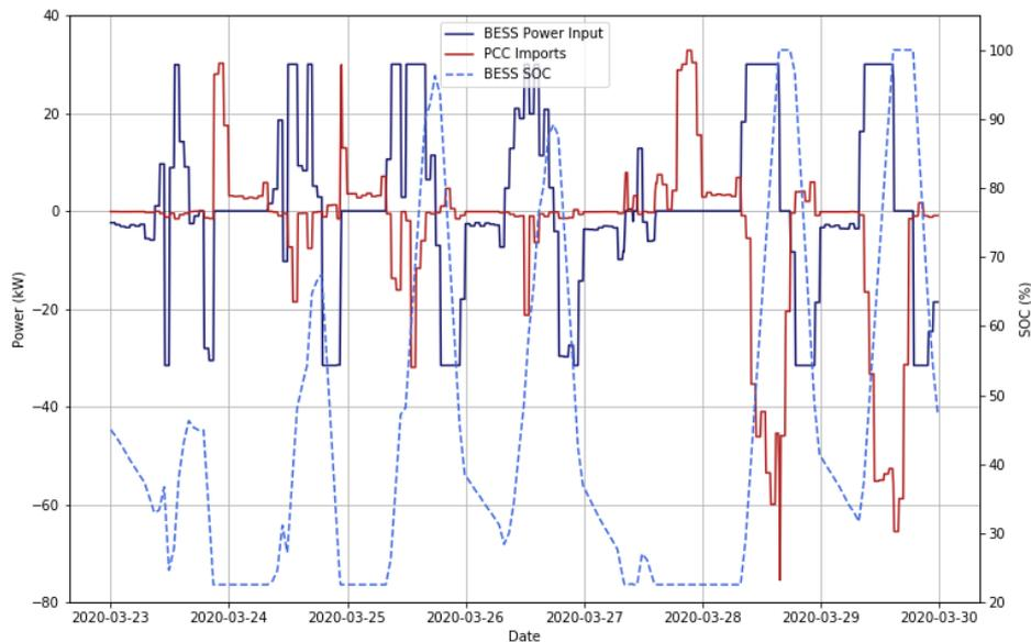
**Figure 6-4. System operation according to EMS optimisation**
