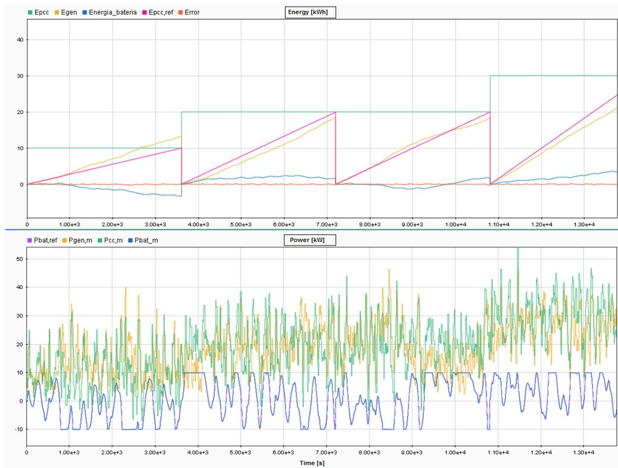
**Figure 3-2. Energy (upper graph) and active power (lower graph) results of the control simulation of the plant during 3.8 hours.**
