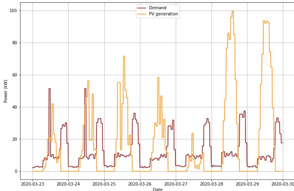
**Figure 6-3. Generation and demand profile used as a reference for the IC validation**
