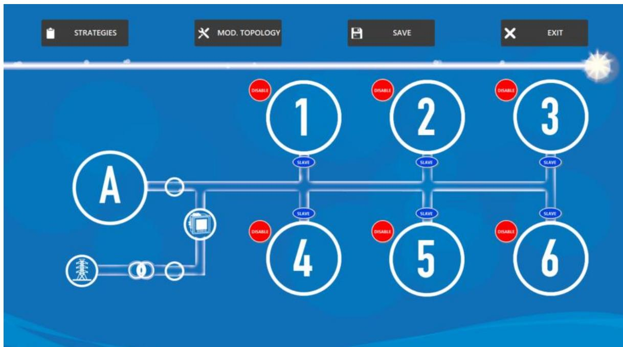
Figure 4-2. Plant configuration screen in the SCADA
