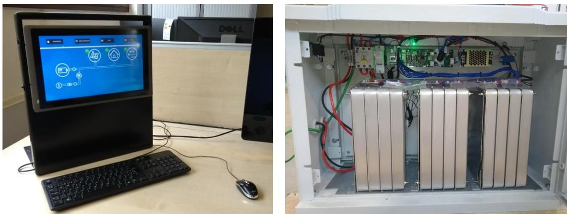
**Figure 6-2. Test set-up: a) HMI-EMS of the IC; b) Test battery.**
