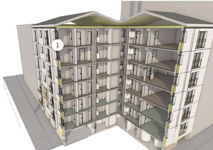
Figure 2: Schematic of the panels including layer for heating and cooling (left) and cross section of the refurbished building (right). Source: Nussmüller Architekten.
